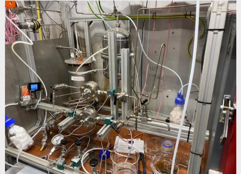
Continuous Flow Reactor 620 °C and 220 bar
